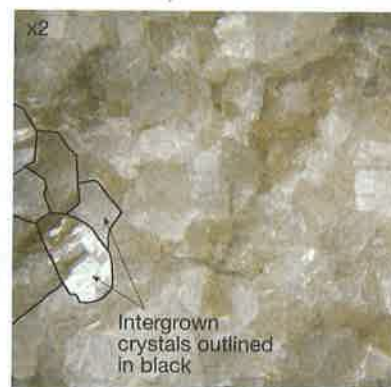
C. Crystal growth of the calcite mineral crystals in this rock (marble) was obstructed in every direction. The crystals grew together as a dense mass of odd-shaped crystals instead of perfect crystal forms.
