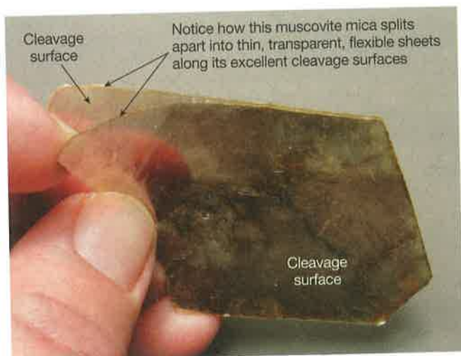
FIGURE 3.13 Cleavage in mica. Mica is a group of silicate minerals that form very reflective (vitreous) tabular crystals with one excellent cleavage direction. The crystals split easily into thin sheets, like pages of a book. This is called book cleavage . Muscovite mica is usually silvery brown in color. Biotite mica is always black.
