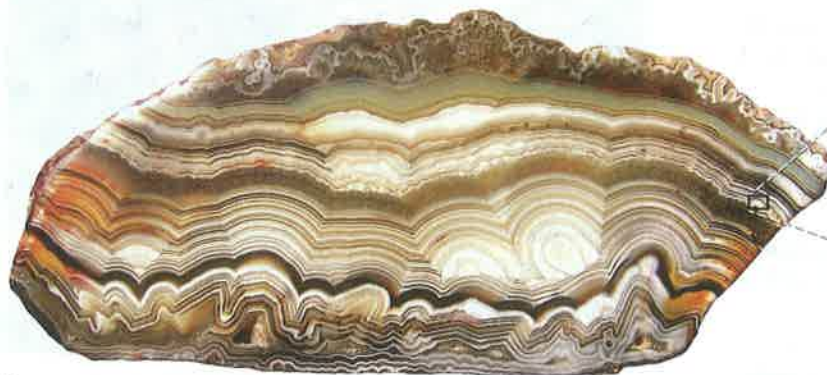
D. Slice of rock (agate) cut with a diamond saw and polished. The layers are made of quartz mineral crystals that are cryptocrystalline (not visible in hand sample). They can only be seen in a thin section (thin transparent slice of the rock mounted on a glass slide) magnified with a microscope to 30 times larger than their actual size (x30).
