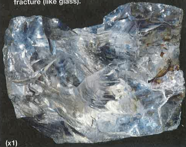
A: Pure quartz (var. rock crystal) is colorless, transparent, nonmetallic, and has conchoidal fracture (like glass).
