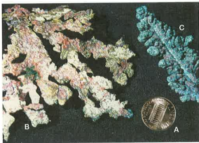
FIGURE 3.6 Native elements. The native elements are minerals composed of just one element, like gold nuggets. A. When freshly formed or broken, native copper (Cu, naturally-occurring pure copper) has a reflective metallic luster like this freshly-minted copper coin. However, these dendritic clusters of native copper crystals have tarnished to nonmetallic dull brown ( A ) and/or green ( B ) colors.
