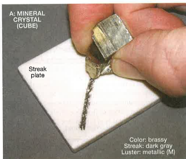
FIGURE 3.7 Streak tests. Determine a mineral's streak (color in powdered form) by scratching it across a streak plate with significant force, then blowing away larger pieces of the mineral to reveal the color of the powder making the streak. If you do not have a streak plate, then determine the streak color by crushing or scratching part of the sample to see the color of its powdered form.
