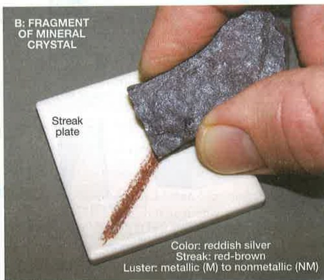
FIGURE 3.7 Streak tests. Determine a mineral's streak (color in powdered form) by scratching it across a streak plate with significant force, then blowing away larger pieces of the mineral to reveal the color of the powder making the streak. If you do not have a streak plate, then determine the streak color by crushing or scratching part of the sample to see the color of its powdered form.
